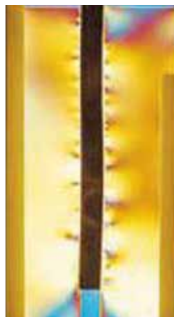
S-shaped stems result in even stress distribution
