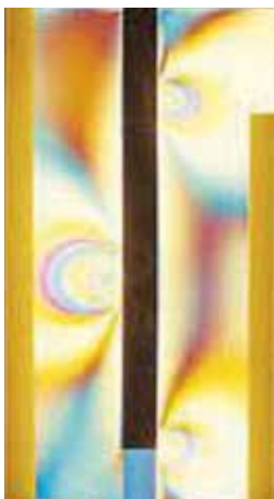
Straight stems produce stress risers in an anatomically S-shaped medullar canal
